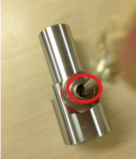
Figure 21 Turning sampling cell valve screw with flathead screwdriver
