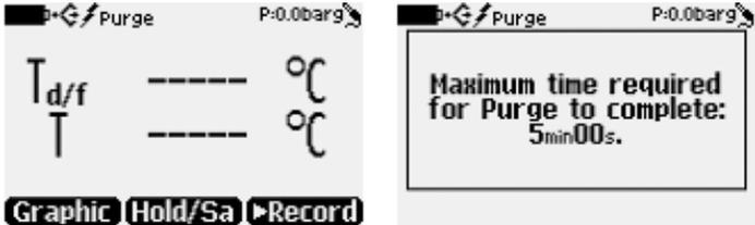
Figure 8 Sensor purge displays
