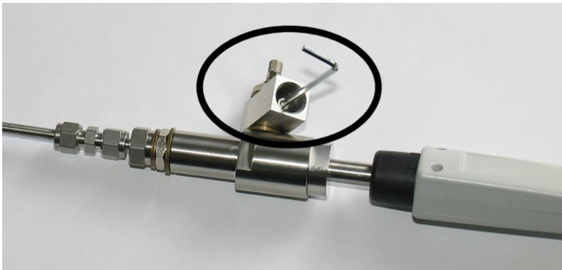
Figure 27 Removing the leak screw
