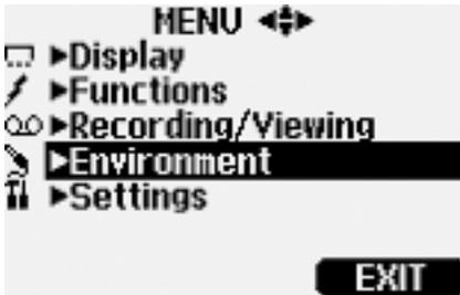
3. To change the pressure unit, press
