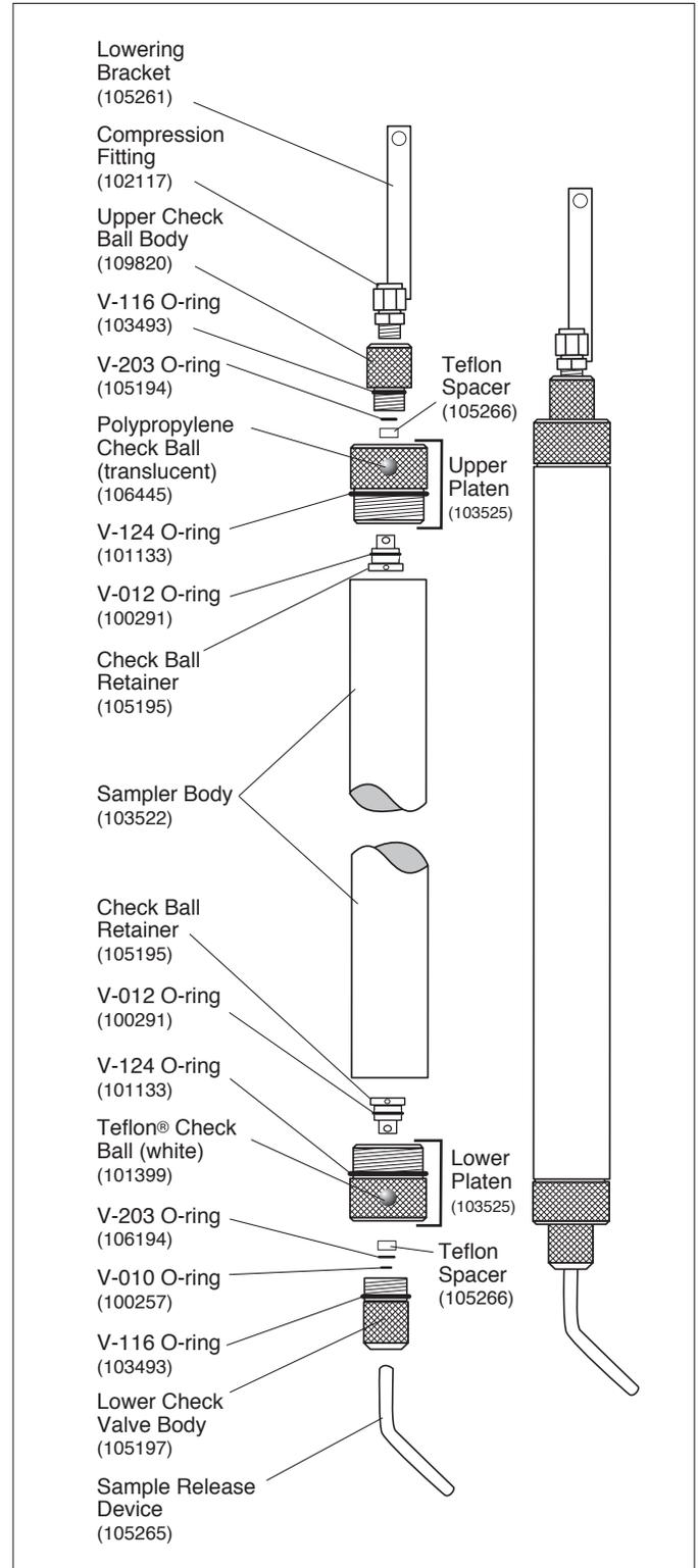
Model 425 1.66" x 2 ft. Discrete Interval Sampler (105264)
