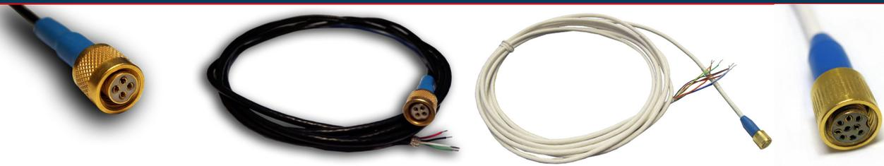
**2240:** The connector shells, pins and sockets are gold plated brass. The 4PIN-CAB cable consists of four 30 AWG (7x38) silver-plated copper wires with PTFE insulation surrounded by a braided shield. The black FEP shield jacket has a nominal outer diameter of 0.100”.
