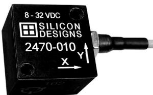
The SDI Models 2470, 2476, 2460 and 2466 are the triaxial aluminum case versions of the 2480. The SDI Models 2470 and 2476 are internally identical to the 2480 with upgraded bias and scale factor temperature shift performance and a wider temperature range from -55 to +125°C. The SDI Models 2460 and 2466 are the three axis low-cost versions of the 2480, rounding out the SDI Universal Module family for lower-temperature applications from -40 to +85°C.
