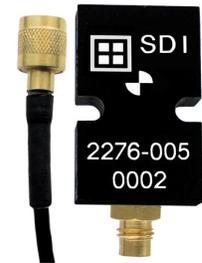
Each SDI single axis accelerometer module features a hermetically sealed low noise accelerometer within a rugged, epoxy sealed, anodized aluminum case. Onboard voltage regulation and an internal voltage reference eliminate the need for precision power supplies. They are relatively insensitive to temperature changes and gradients. The case is easily mounted via two screws, an adhesive, or by attaching a magnet.
