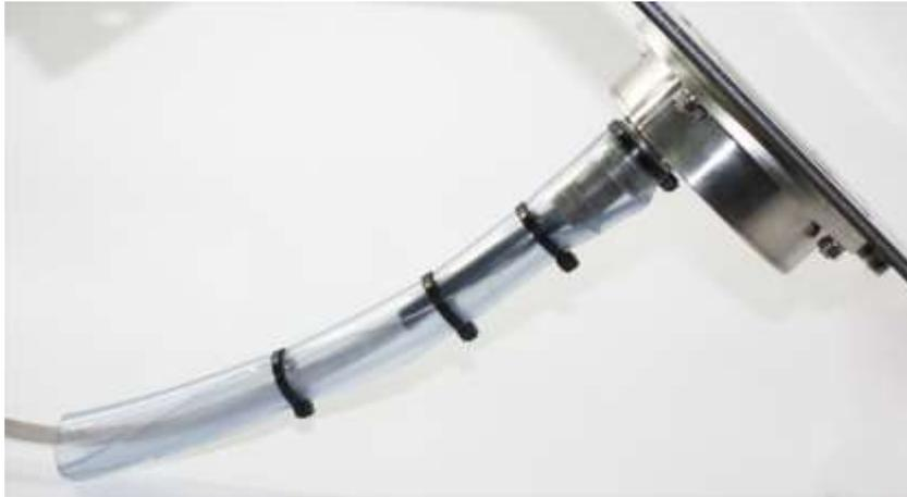
Alternatively, the included shrink sleeve over the cable can be used. After installation of the SONO-probe and connection of the MIL-connector, the shrink sleeve can be shrunk with a hot air blower.
