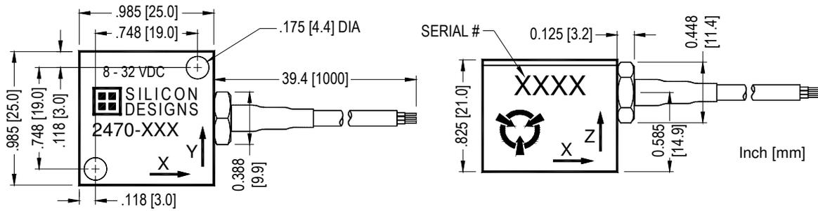
**Note:** The cable's braided shield is electrically connected to the case. The black ground (GND) wire is isolated from the case.
