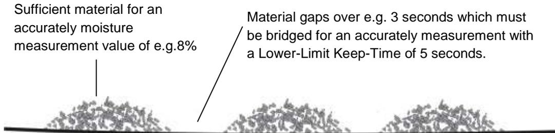
The following parameter setting in mode CA fits a high pass filtering for bridging material gaps.
