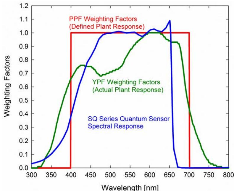
Radiation weighting factors for PPFD (defined plant response to radiation), YPF (measured plant response to radiation), and Apogee quantum sensors (sensor sensitivity to different wavelengths of radiation).
