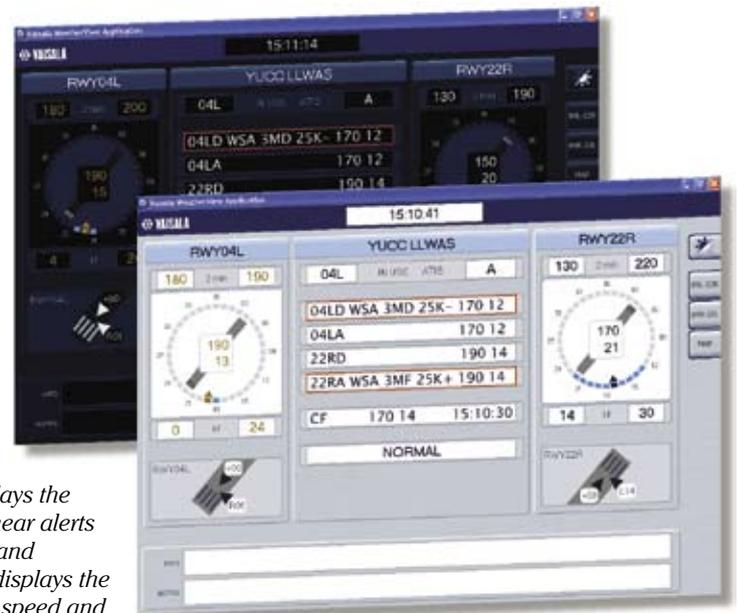
*Alert screen displays the threshold windshear alerts and wind speed and direction. It also displays the center field wind speed and direction and system status.*
