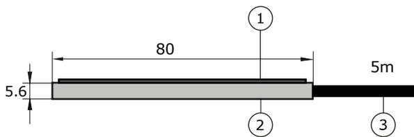
**Figure 3** HFP01SC self-calibrating heat flux plate: (1) film heater, (2) heat flux sensor plus passive guard, (3) 2 x cable, standard length is 5 m (optionally longer cable). Total sensor thickness including heater and covers is  $5.6 \times 10^{-3}$  m ( $6 \times 10^{-3}$  m at cable exit from sensor). Dimensions in  $\times 10^{-3}$  m.
