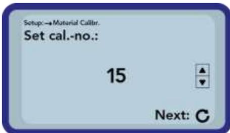
First you have to set the calibration curve to be changed (01 – 15) by pressing the buttons „Up“
