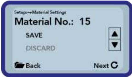
Finally you can store the calibration into the chosen calibration storage inside the probe. Choose „SAVE“ and confirm by pressing the button „Measurement“
