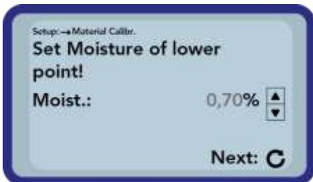
Next set the moisture of the lower moisture point by pressing the buttons „Up“
