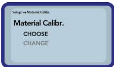
After the selection of the menu item „Material Calibration“, you have to choose between “CHOOSE”, to save one out of fifteen calibration as default calibration, or “CHANGE”, to setup a new calibration in one of the fifteen calibration storages
