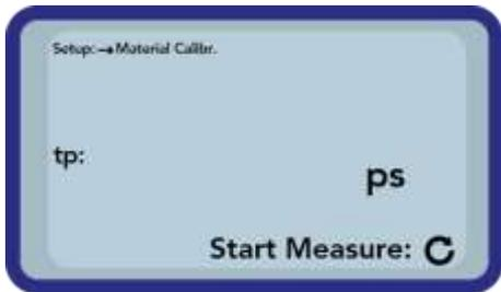
To start the measurement push the button „Measurement“ . To increase the accuracy four measurements take place. The whole time of measurement is about 20 seconds. Afterwards the measured average impulse duration is shown for a short moment.
