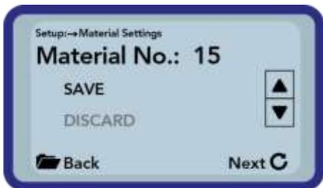
Finally you can store the calibration into the choosen calibration storage inside the probe. Choose „SAVE“ an confirm by pressing the button „Measurement“ . If you choose “DISCARD” everything is left untouched.
