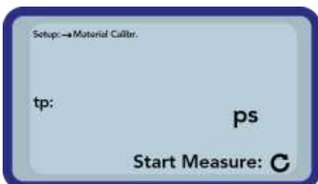
To start the measurement push the button „Measurement“
