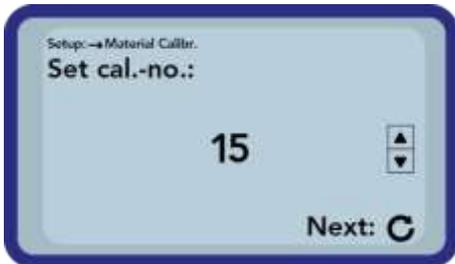
First you have to set the calibration curve to be changed (01 – 15) by pressing the buttons „Up“
