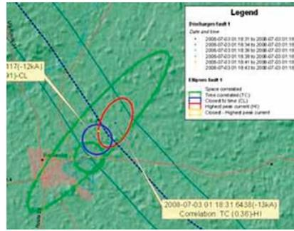
*This FALLS® Reliability Analysis reveals four cloud-to-ground lightning discharges which correlated to a suspected fault. The blue ellipse represents the stroke that best matches the fault recorder time-stamp and the red ellipse shows the highest peak current event. Field crews could be dispatched to the location to restore service.*
