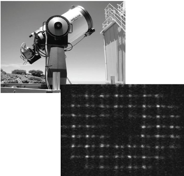
Slope Detection and Ranging (SLODAR) double star technique using the 860 model with 2 ms exposure time. The camera is shown at the European Southern Observatory (ESO) site at Cerro Paranal in Chile, mounted on a 40cm Schmidt-Cassegrain telescope and operated through Linux. The image shows an example Shack-Hartmann wavefront sensing frame.
