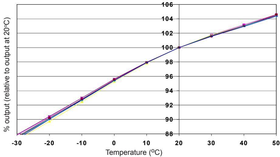
Figure 2 shows the very repeatable variation in sensitivity caused by changes in temperature.
