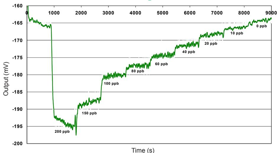
With a 33 Ω load resistor, the NO<sub>2</sub>-B42F shows excellent resolution, even at the ppb level: ideal for outdoor air environmental testing.
