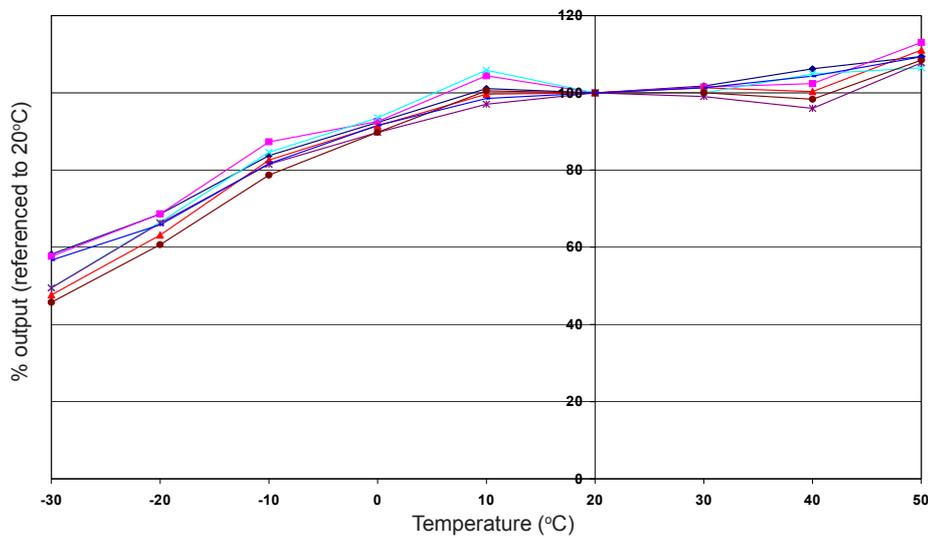
Figure 2 shows the temperature dependence of sensitivity at 2ppm NO<sub>2</sub>. This data is taken from a typical batch of sensors.
