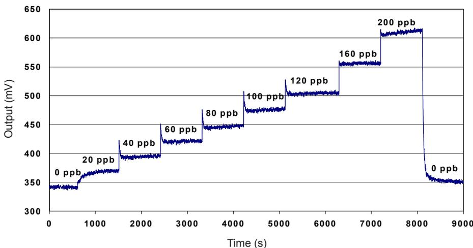
Figure 4 shows response to 200ppb H<sub>2</sub>S.
