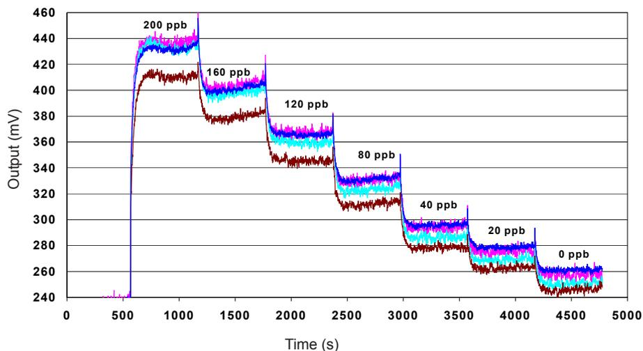
Figure 4 shows response to 200ppb H<sub>2</sub>S.
