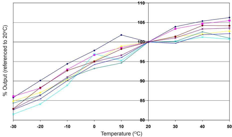
Figure 2 shows the temperature dependence of sensitivity at 2ppm H<sub>2</sub>S.
