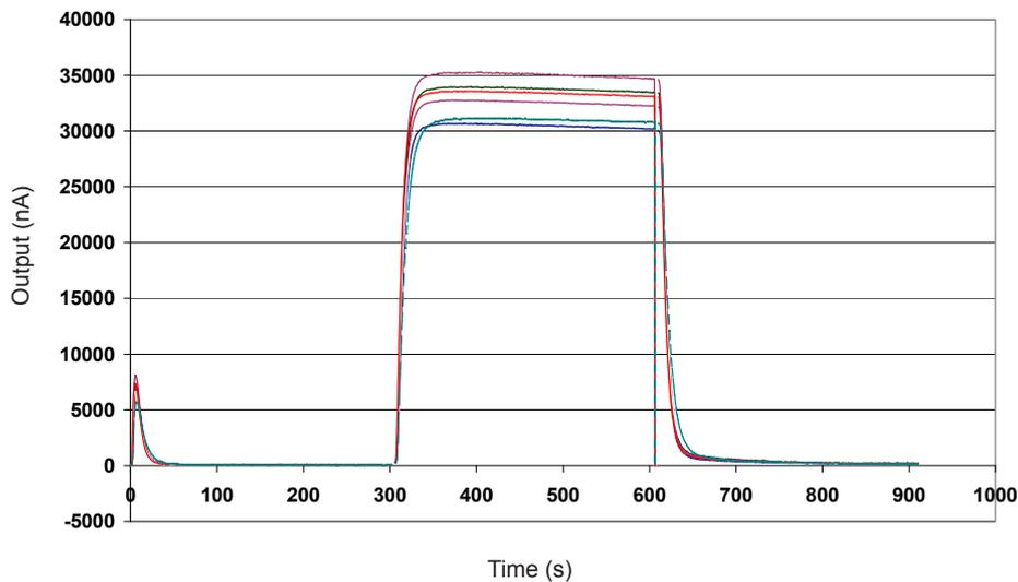
Figure 3 shows the response for a batch of sensors tested with 400ppm CO. The fast, stable response shows a robust sensor that operates well above its specification.
