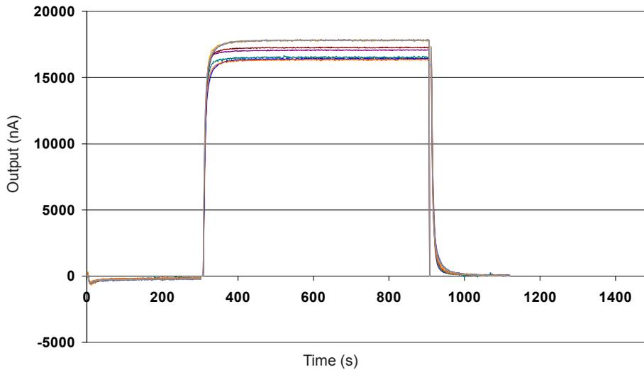
Figure 5 shows response to 25ppm H<sub>2</sub>S. Sensor shows a fast and stable response and recovery and repeatable sensitivity.
