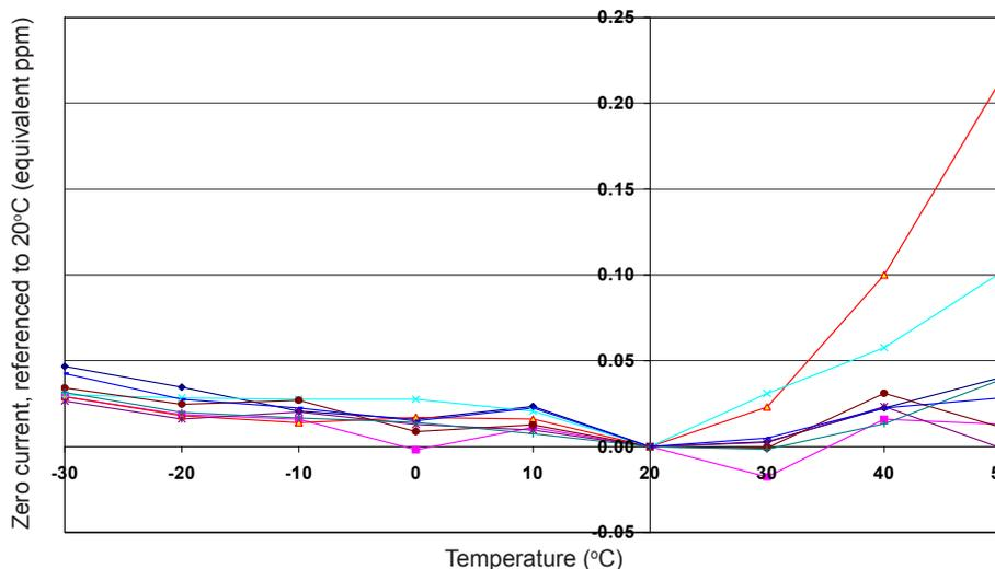
Figure 7 shows the variation in zero output caused by changes in temperature, expressed as ppm gas equivalent, referenced to the zero at 20°C.
