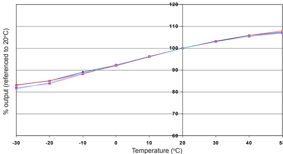
Figure 6 shows the % variation in sensitivity caused by changes in temperature.
