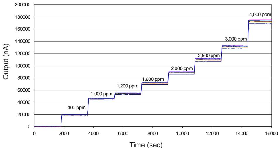
Figure 4 shows sensor output for increasing concentrations of CO, up to twice the specified overgas concentration. Data shown is eight sensors taken from a typical production batch.
