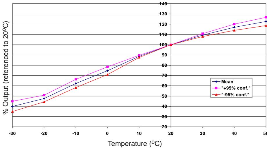
Figure 2 shows the variation in sensitivity caused by changes in temperature. Repeatable temperature dependence at elevated temperatures allows more accurate temperature compensation.
